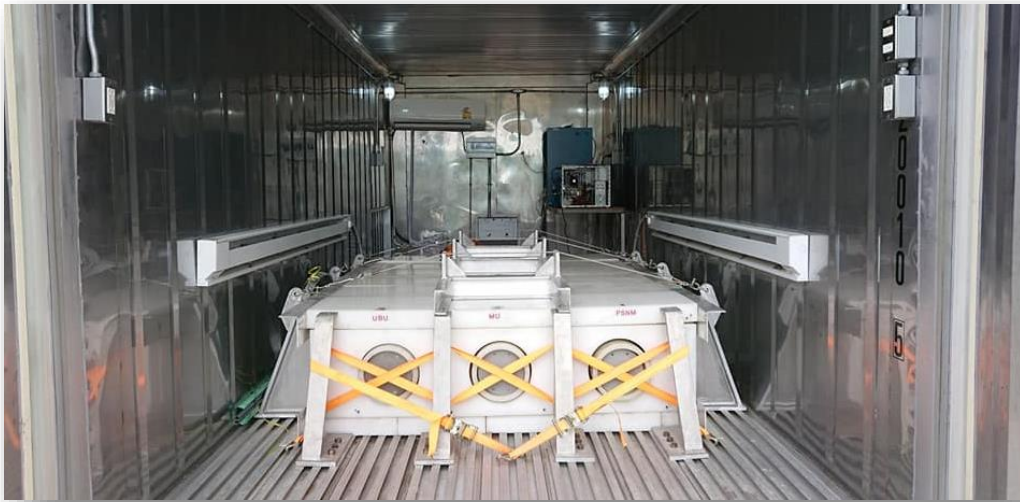
FIGURE 17 The placement of the 2NM64 and semi-leaded neutron detectors inside the Changvan Courtesy Khampakdee et al.
