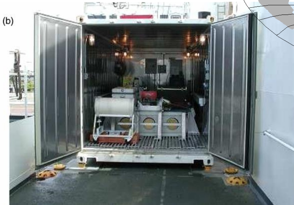
Fig 8. 3NM64 installed inside the container for latitude survey (Nuntiyakul et al., 2014)
