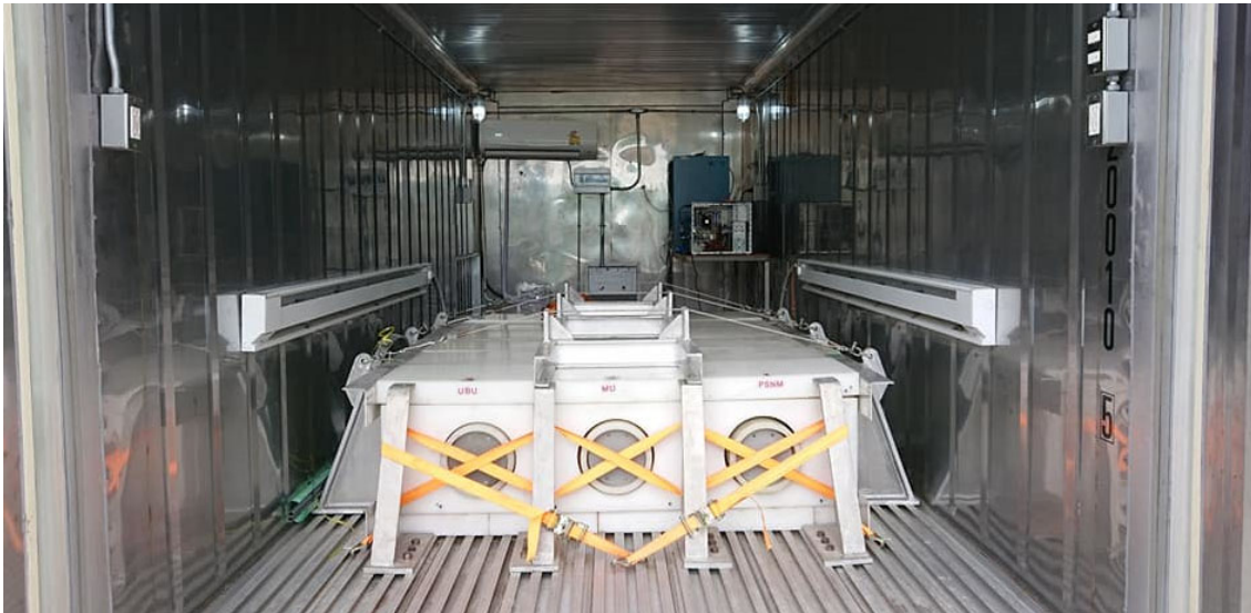
FIGURE 18 The placement of the 2NM64 and semi-led neutron detectors inside the Changvan.
