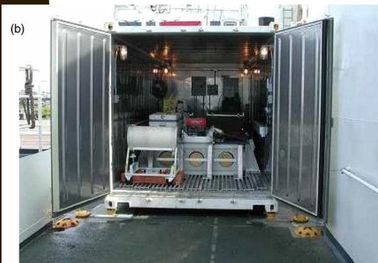
Fig 8. 3NM64 installed inside the container for 1994-2007 latitude survey (Nuntiyakul et al., 2014)
